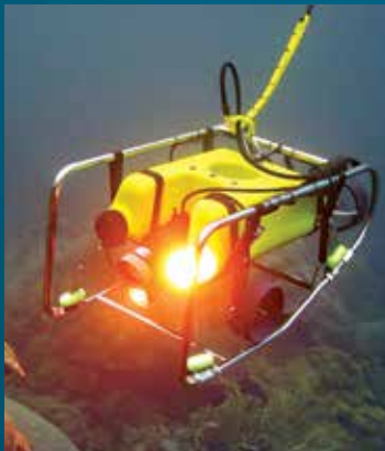
Both National Geographic Explorer and Orion are also equipped with an ROV (Remotely Operated Vehicle) capable of exploring depths up to 1,000 feet, well beyond the limits of our human divers.
